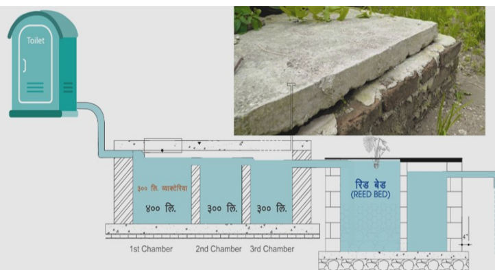
Detailed technical drawing of bio-digester plant and the constructed septic tank (PC: Birendra Shahi, NRCS, HQs)
