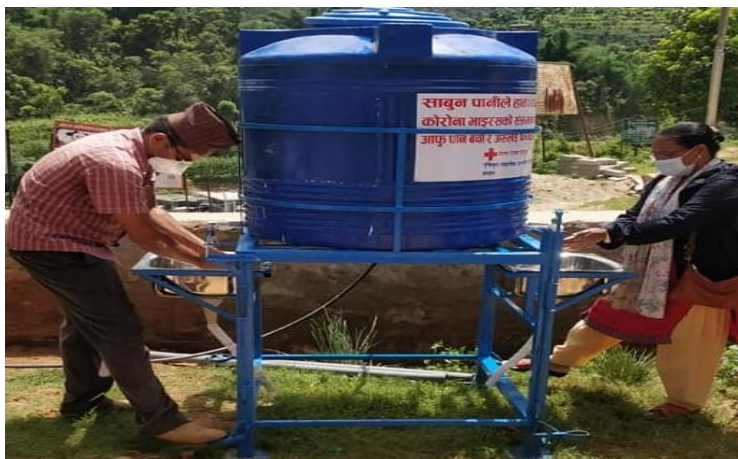
Figure :Contactless handwashing station in Salyan district.
